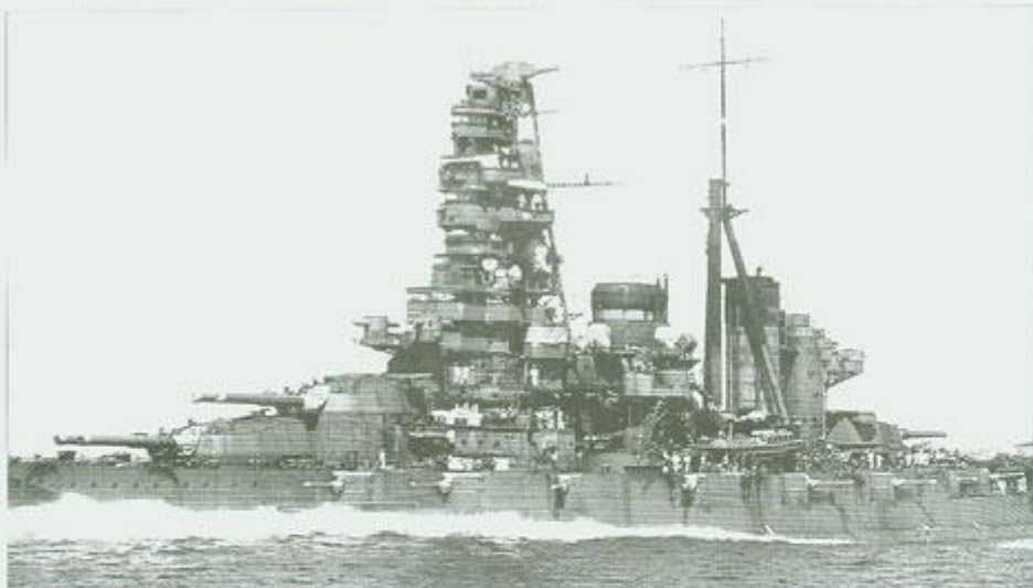
Midship of BC Haruna in 1928 (upper) after the first modernisation conversion and 1934 after the second one. Pay attention to the reversion of the height of the funnels beside of noting the complete revisions of foremast and after superstructure.
