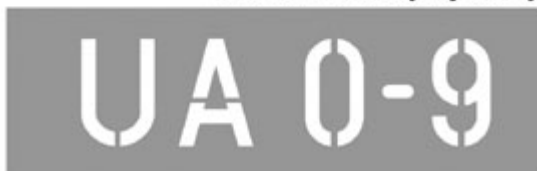
Oznaczenia o wys.ok.80mm malowane na drzwiach po obu stronach pojazdu, wg. zasad podanych na drugiej stronie Small registration numbers ( ca. 80mm height ) had been painted on the both sides of vehicle, on the truck's door - see rules at the opposite site
