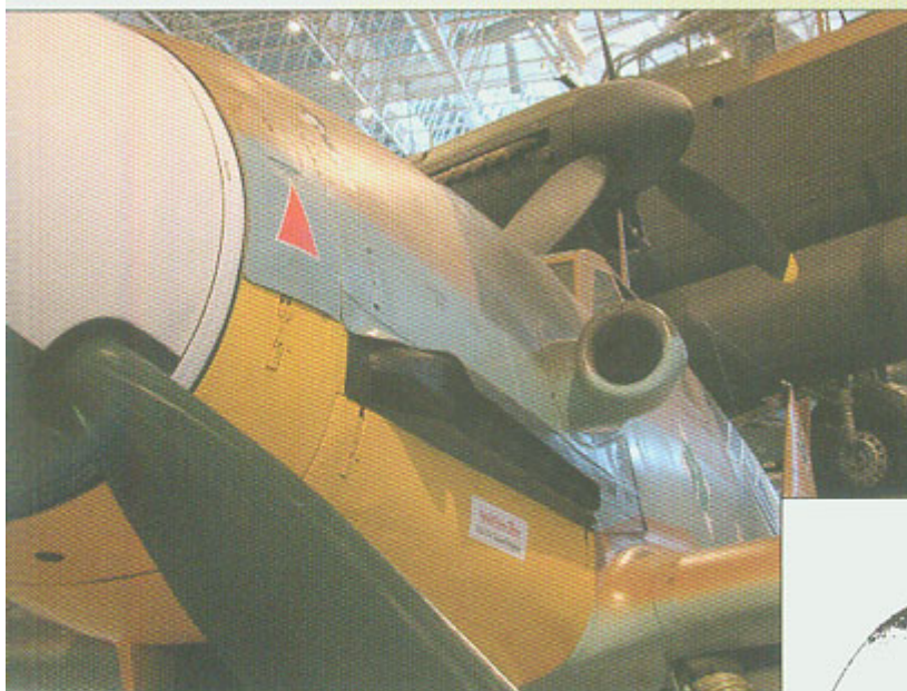
Port side of the engine cowling. Note the shape of the supercharger intake – Bf 109F-4/Z.
