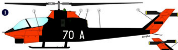
TH-1G s/n 34276, 70 A One of trainer Cobras of US Army. Standard cammo scheme with areas of International Orange outline, usual for trainer helicopters. Cobas 70 A in white, serial number and other inscriptions in Black.
