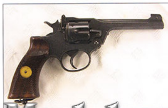
The Pistol Enfield No 2 Mk I* - note the lack of a hammer spur.
