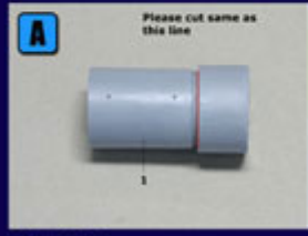
(A) Burner pipe
