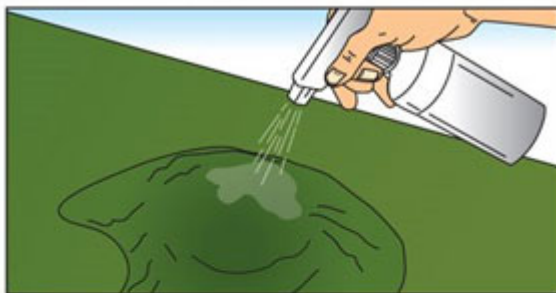
Spray adhesive on area to be landscaped.
