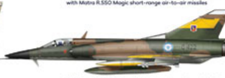
IAI Dagger, "C-422", Fuerza Aerea Argentina, Grupo 6 de Caza, Rio Grande or San Julian airfield, April/May 1982. The plane is wearing yellow fast id markings on vertical stabilizer, upper surfaces of the wing and lower surfaces of drop tanks
