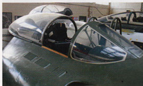
A quick close-up of the 'clear' canopy used on the FR Mk 5, as seen here on the RAF Museum example at Tangmere (©J. Mills)
