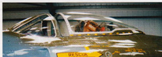
A quick close-up of the 'clear' canopy used on the FR Mk 5, as seen here on the RAF Museum example at Tangmere (©J. Mills)
