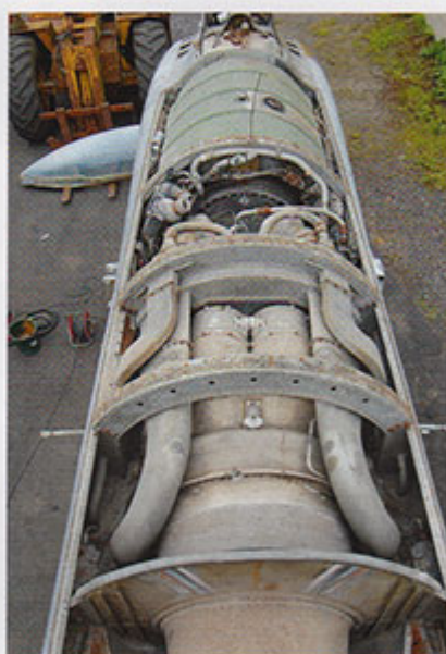
This is the Avon being removed from the fuselage of F Mk 4 WK275 during the initial dismantling prior to restoration (©Jet Art Aviation Ltd)
