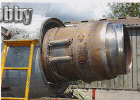
This is the afterburner nozzle in the back of F Mk 4 WK275 during strip-down (©Jet Art Aviation Ltd)
