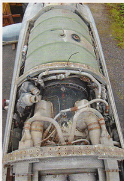
Here is a close-up of the front section of the Avon along with the fuel cell in front of it; the front of the aircraft is at the top of this image (©Jet Art Aviation Ltd)
