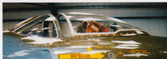
A quick close-up of the 'clear' canopy used on the FR Mk 5, as seen here on the RAF Museum example at Tangmere (©R. Mills)
