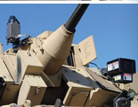
FIG 45 Close-up of a turret attachment for a part of the M2E1 gun. FIG 46 A shot of the front of the turret, showing the sensor for the M2E1 gun and the gun attached.
