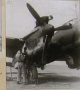
(115) An UPe-2 with engines differing from each other in the exhaust systems. The starboard engine has exhaust manifold, while the port one had individual exhaust stacks.
