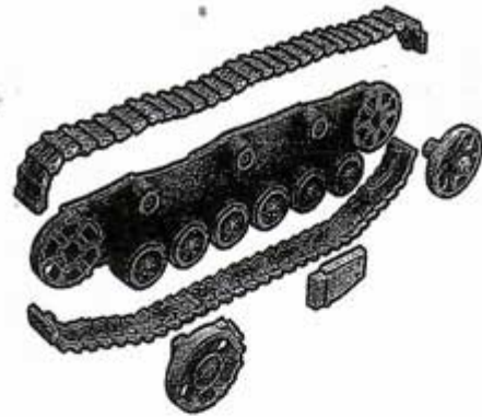
2. Running gear sub-assembly
