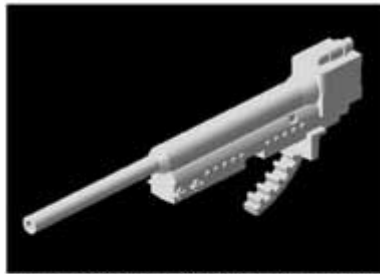
● One-piece 3.7cm PaK with hollow muzzle made by side mold
