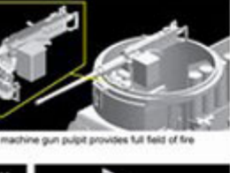
• Newly designed M2 machine gun pulpit provides full field of fire
